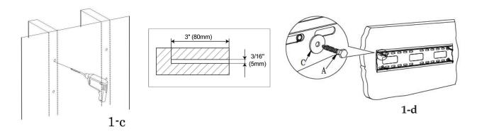
**CAUTION**: Do not over tighten the bolts - doing so may cause unnecessary damage to the wall. Avoid excessive torque.
